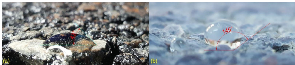
Fig. 1. Contact angles of water on (a) uncoated and (b) SH coated surface.
