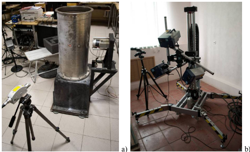
Fig. 1. a - Polytec® OFV-534 vibrometer; b - Polytec® PSV-400-3D scanning vibrometer
