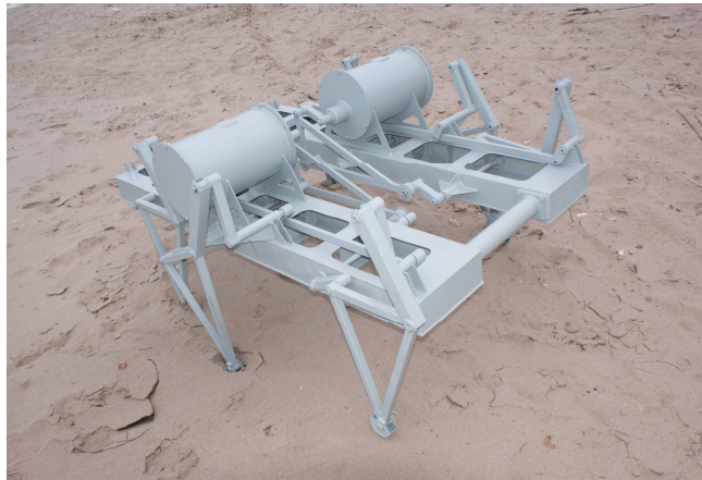
Fig. 1. Walking machine MAK-1
