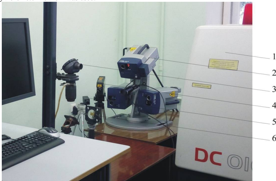
Fig. 1. A general view of the experimental stand for studying the vibration characteristics of objects during the laser-induced nanopores formation: 1 - CO 2 -laser ROFIN DC 010 with a diffusion-cooled high-frequency pumping; 2 - three-axis scanning laser vibrometer Polytec® PSV-400-3D; 3 - optical system; 4 - Polytec PDV 100 two-coordinate measuring instrument; 5 - non-contact thermometer "Kelvin LCM-1300"; 6 – the sample of brass L62.
