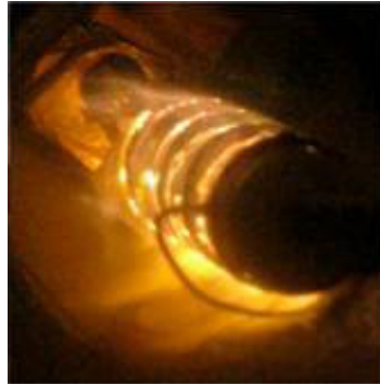
Fig. 1. Integral image of the rotating electric arc on the surface of the cylindrical model.
