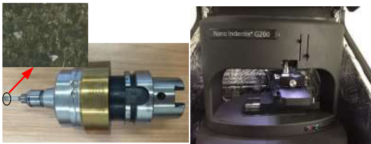
Fig. 1. The tool with its 1000X photos and the nano indenter
