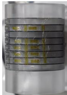
Fig. 2 Installation of strain gauge
