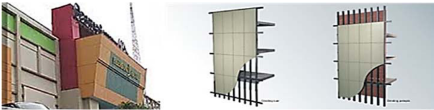
Fig. 1. Calcium silicate board uses as façade and room partition
