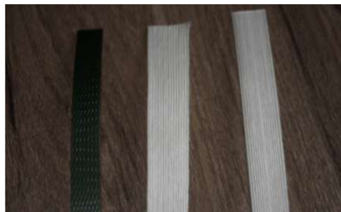
Fig. 1 From left to right PET, glue bonded polyester and PP coated polyester straps
