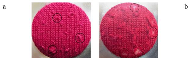
Fig. 1. Stage of abrasion test: (a) First stage – small balls entanglement; (b) Second stage – holes apparition.
