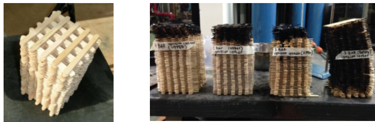
Fig. 1. Wood cribs as source of fuels in this experimental work.
