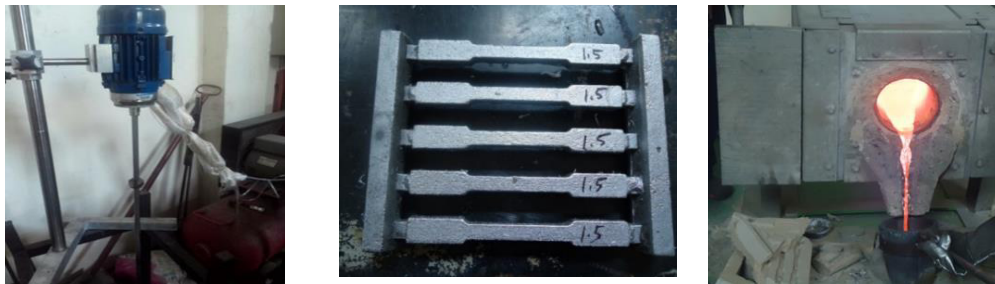
Figure 1. Preparing composite by Vortex method
