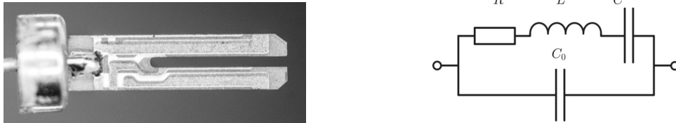
Fig. 1. (a) Commercial off-the-shelf 32.768 kHz clock crystal (~2 x 7 mm) with removed housing; (b) Butterworth - Van Dyke model for QCR. The simple damped resonant circuit is paralleled by the electrode capacitance C_0 of the QCR.
