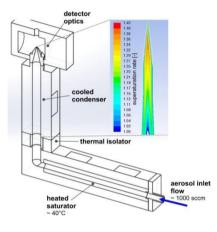
Fig 1: Fundamental CNC sensor layout.
