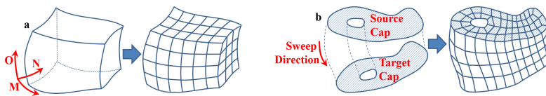
Fig. 2. Block types used in Mesh Scaling. a) a structured block. b) a swept block.
