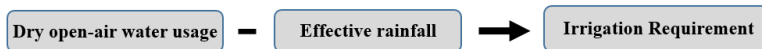
Fig 1. The irrigation requirement of a particular crop is determined by factoring in average daily rainfall to its daily open-air water usage. Adapted from FAO Irrigation Water Management Training Manual [7].
