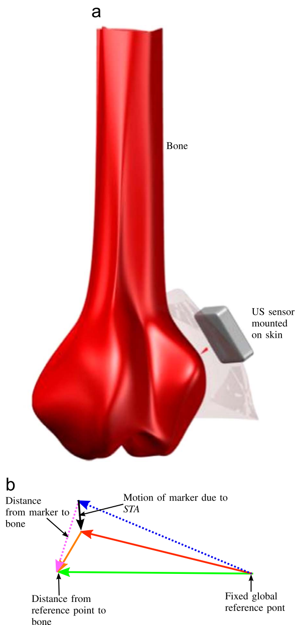
Fig. 1. (a) US sensor attached to the skin, (b) Illustration of the concept for STA compensation. (For interpretation of the references to color in this figure, the reader is referred to the web version of this article.)
