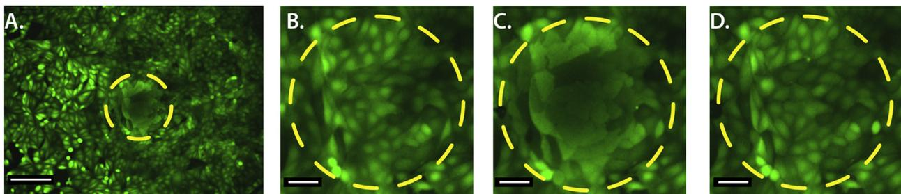
**Fig. 2.** (A) MDCK monolayer under persistent 50  $\mu\text{N}$  load. Scale bar: 200  $\mu\text{m}$ . Monolayer indentation viewed at higher magnification, before (B), during (C), and after indentation (D) is performed without apparent cell damage. Scale bar: 50  $\mu\text{m}$ .
