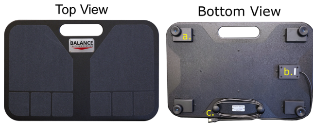
Fig. 1. Top (left) and Bottom (right) views of the BBP. Labelled are a) one of the four enclosed sensors in the plate corners, b) the enclosed bridge-type circuit board, and c) the USB connector for interfacing with a computer.
