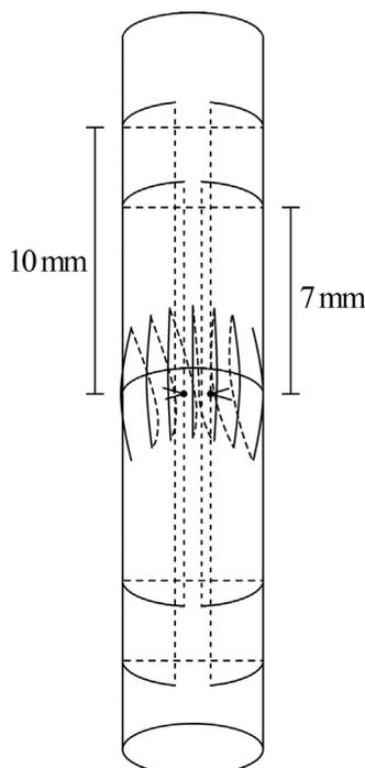
Fig. 1. A schematic illustration of the repair method.
