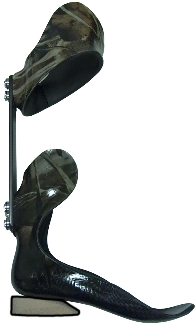
Fig. 1. The Intrepid Dynamic Exoskeletal Orthosis (IDEO) is a novel, semi-rigid ankle-foot orthosis that was developed to improve functional outcomes of service members with traumatic musculoskeletal lower extremity injuries. The IDEO is comprised of: (1) a proximal cuff that off-loads the injured limb, (2) a posterior carbon fiber strut that stores and returns energy, (3) a cushioned foam heel wedge that softens the impact and aids in placing the device in a toe down position, and (4) a foot plate that provides a lever to allow deformation of the posterior strut and provides control of frontal plane foot motion.
