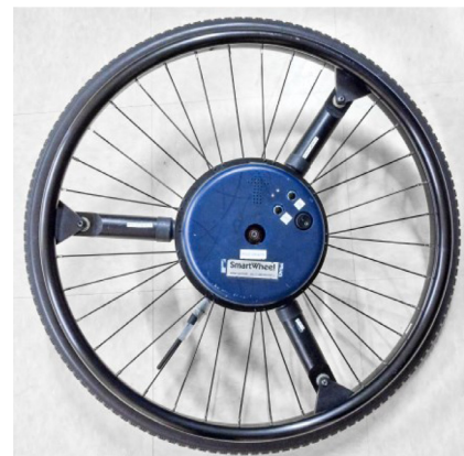
Fig. 1. The SmartWheel™ instrumented wheel.
