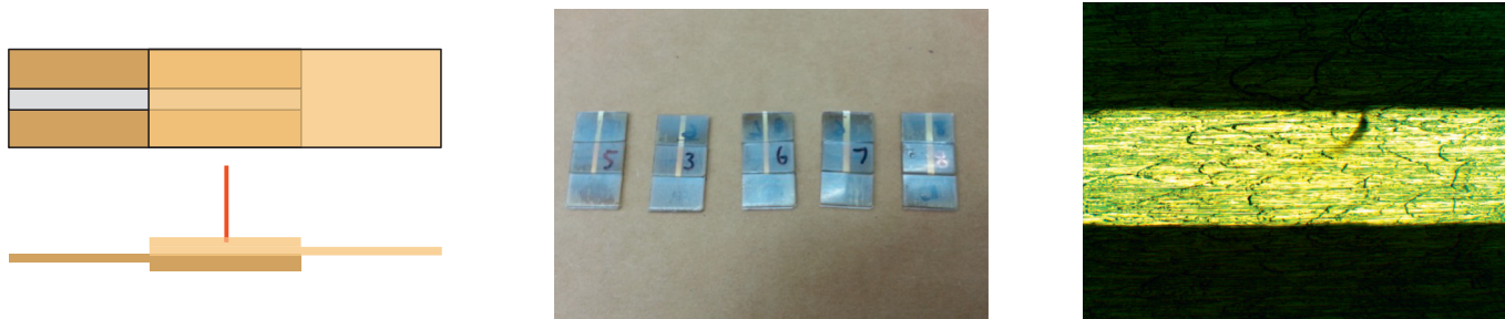
Fig. 1. PEEK strips. Left: top-view (top) and side-view (bottom) schematic of PEEK strips consisting of a base layer containing Lumogen on which silver tracks have been sputtered, and a PEEK layer laser-welded on top. Middle: PEEK strips after laser joining. Right: microscope image of sputtered Ag track on PEEK substrate.
