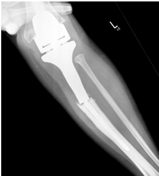
Fig. 1. X-ray of fractured stem showing fracture at the shoulder of an implant with no evidence of bone ingrowth for tibia in lower leg.
