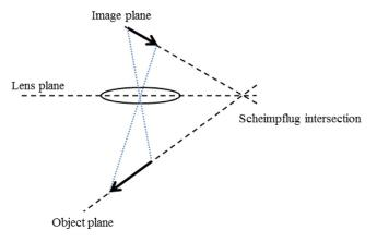
Fig. 1. Illustration of the Scheimpflug principle.
