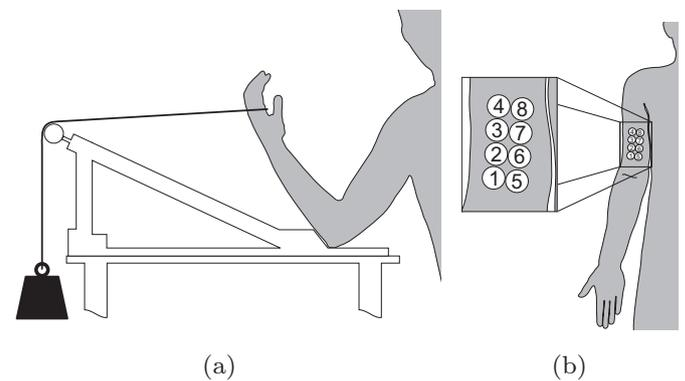
**Fig. 1.** Setup of the experiment (drawing adopted from [12]). The block and pulley construction is shown in (a). The seated subject was asked to hold his/her arm in a bent position (approximately 90° between upper and lower limb) keeping the weight suspended. (b) shows the positions of the electrodes on the subject's biceps. Electrodes 3 and 7 were placed above the thickest point of the biceps whereas electrodes 1 and 5 were placed on the distal end of the upper arm.
