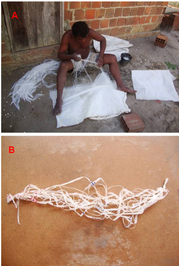
Fig. 1. Crab harvester shredding polypropylene bags for making the tangle-netting (A) and a tangle-netting manufactured in Tramataia community - PB (B). Photos: Douglas Nascimento.
