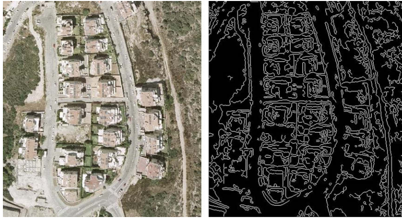
Fig. 1. An orthophoto map of a typical residential area (left); extracted edges (right).
