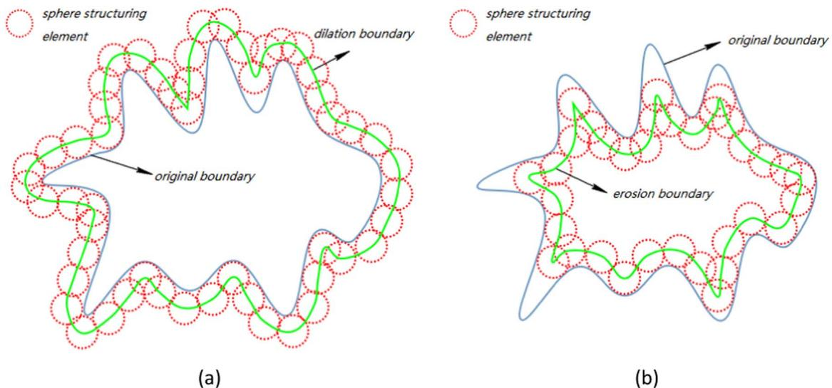
Fig. 1. Brute-force algorithms for dilation and erosion: (a) dilation; (b) erosion.
