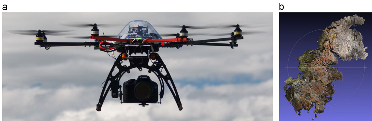
Fig. 1. (a) Oktokopter Micro-UAV, fitted with Canon 550D digital SLR Camera. (b) Densified point cloud generated from UAV images using photogrammetry.
