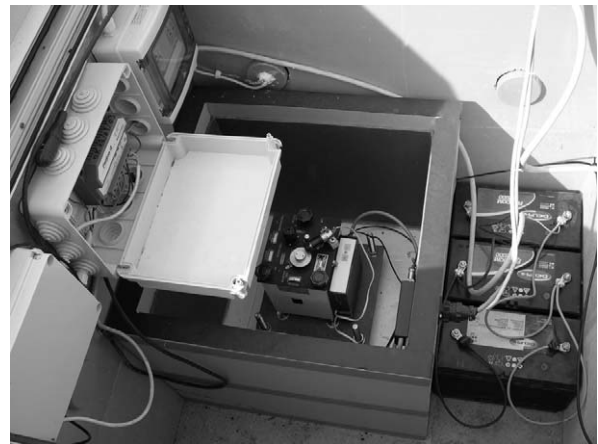
Fig. 2. Set-up of a gravity station on Etna.
