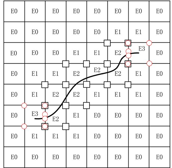
Fig. 1. A typical finite element mesh with an arbitrary crack for the X-SBFEM.
