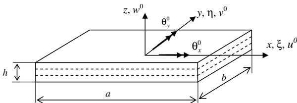
Fig. 1. Plate dimensions, displacements, global and local (*ξ* and *η*) coordinates.
