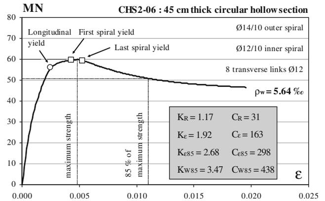
Fig. 1. Typical capacity curve of a circular hollow section model (CHS-06).
