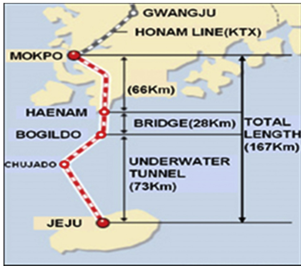
Fig. 1. Concept of Mokpo and Jeju high-speed rail. Source: The Jeju weekly, 4. January, 2010.
