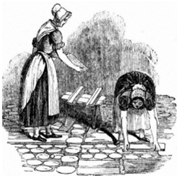
Fig. 1. Women preparing the successive layers of manure, clay jars of vinegar, sheets of lead, and boards, following the Dutch method of producing white lead [13].
