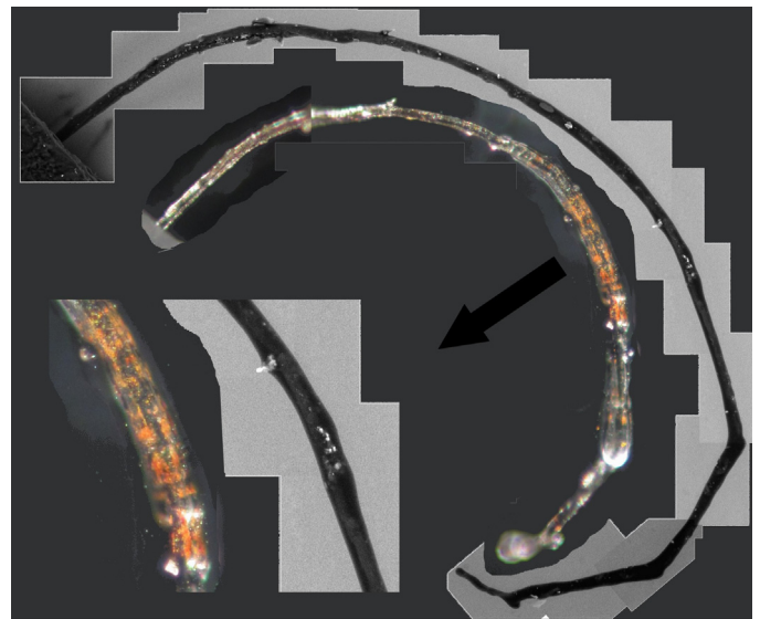
Fig. 1. Fiber 1 of 1HB sticky tape seen with its zoom on the bottom left, by means of both an optical microscope and an ESEM-BSE Detector. While both the blood particles and the inorganic SMP appear reddish in the optical microscope, the inorganic ones appear almost white in the photo obtained using an ESEM-BSE Detector and the blood particles appear dark grey, thus allowing to distinguish the organic from the inorganic particles.
