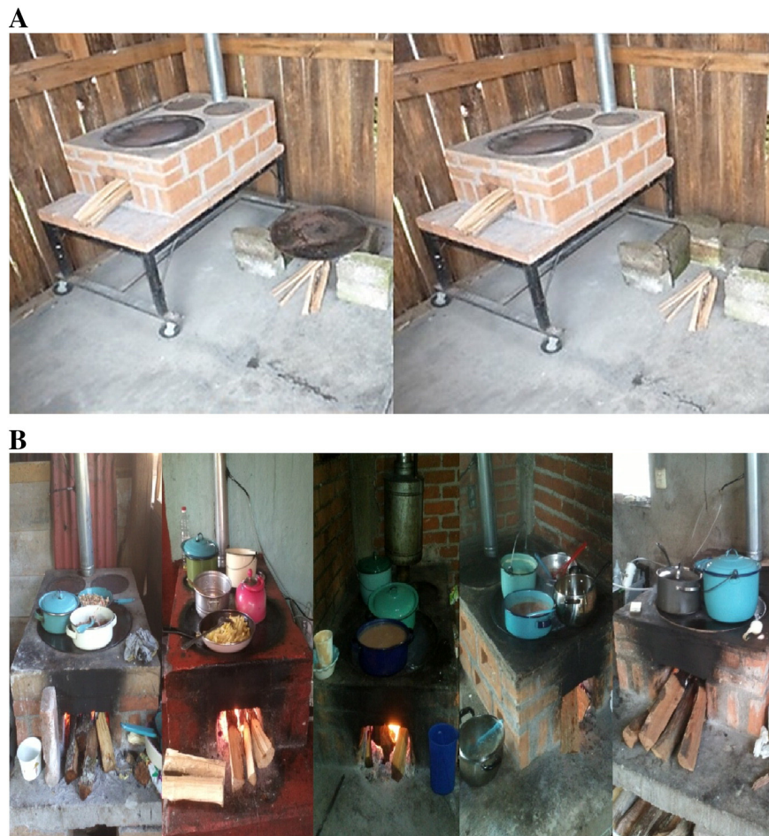
Fig. 1. A. Stoves tested. Left to right: Patsari stove and the U-type. B. Different in-field simultaneous cooking of several dishes on Patsari stoves observed in Purepecha Region of Central Mexico.
