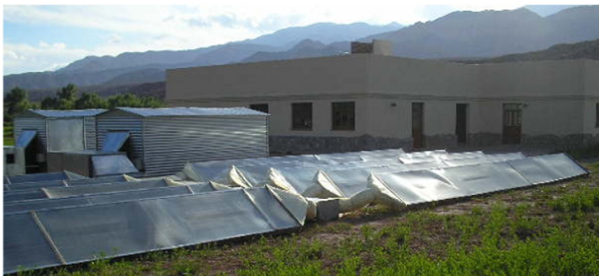
Fig. 2. Photograph of solar dryer. The collector array, fan cabinet and drying chamber are shown.
