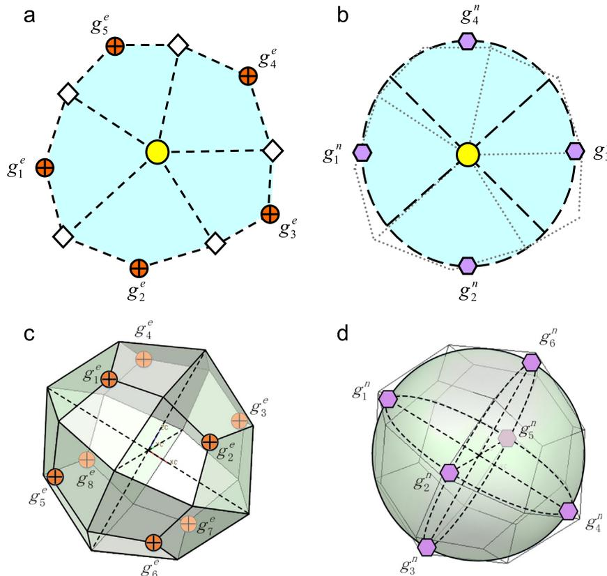
Fig. 2. The integration domain and integration points for FEM and SNIM-SG for 2D and 3D problems. (a) FEM integration for 2D, (b) SNIM-SG integration for 2D, (c) FEM integration for 3D, and (d) SNIM-SG integration for 3D.
