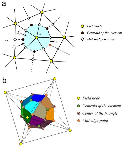
Fig. 1. The schematic of a node-based smoothing domain for node  $k$ . (a) 2D smoothing domain, and (b) 3D smoothing domain.
