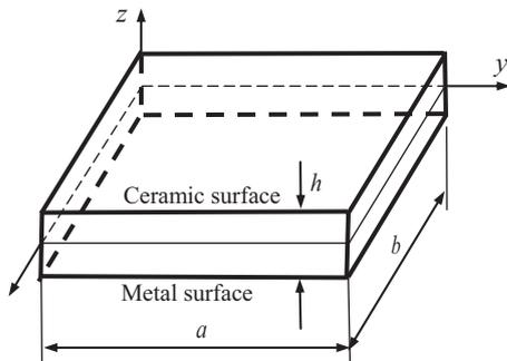
Fig. 1. Sketch of functionally graded plate.
