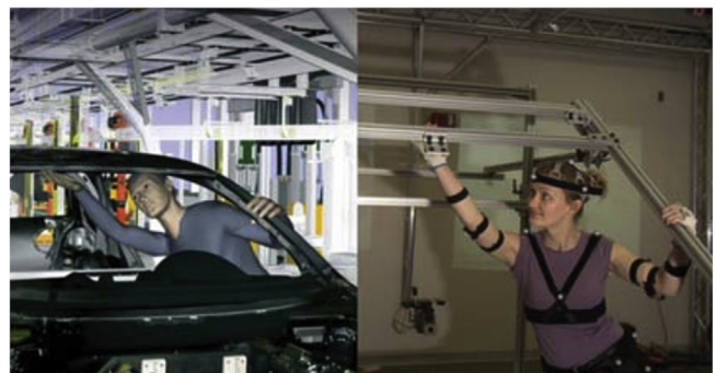
Fig. 2. Animation of a DHM using motion capture data, with the Jack software (picture from Jack documentation). The human subject is placed in a physical mock-up of the environment in order to obtain realistic motions.
