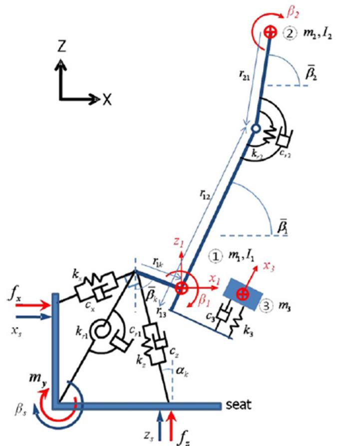
Fig. 1. A schematic view of the five degrees-of-freedom model of the seated human body.
