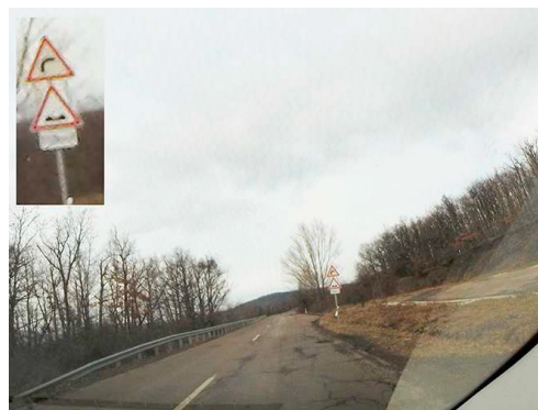
Fig. 1. A bending road in the Mátra Mountains. The drivers are forewarned of the sharp turn of the road by the bend to right traffic sign. In the inset, the two distant traffic signs appear enlarged.
