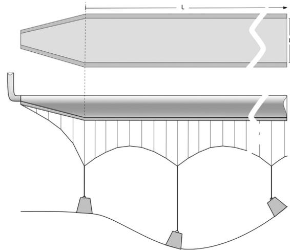
**Fig. 1.** A flat rectangle is curved and the two long sides are sewn together. The ends are capped of by reducing the section progressively. The length of the ropes compensate for small scale unevenness of the ground.
