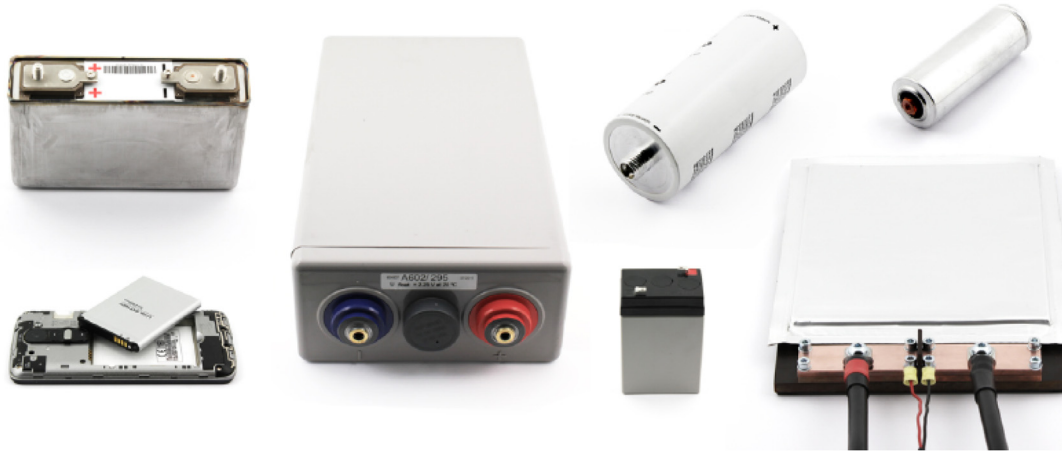
Fig. 1. Exemplary selection of battery cells with terminals for press contacts.
