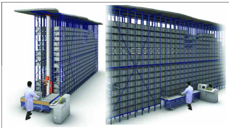
Fig. 1. Picking zone positions in a miniload AS/RS. Both end of aisle (left) and outboard side (right).
