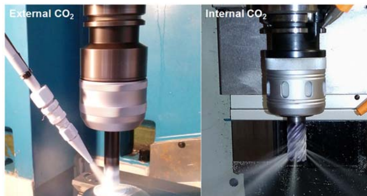
Fig. 1. CO 2 injected as external and internal coolant.
