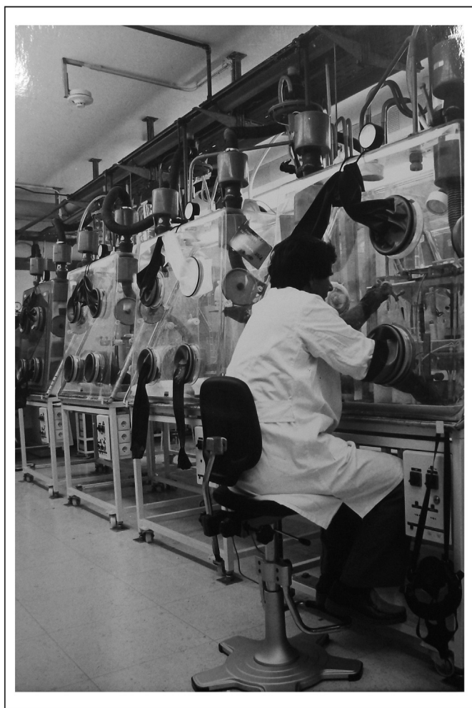
Figure 1. Shown is a series of glove boxes, which permit gram quantities of plutonium to be processed for analysis at the IAEA's Safeguards Analytical Laboratory, 1985. (Courtesy of the Archives of the International Atomic Energy Agency, no. A0739).
