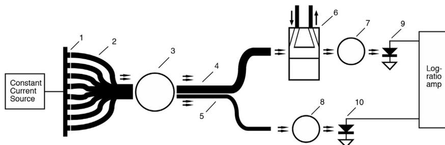
Fig. 1. Schematic drawing of the design of the detector (not to scale): (1) UV-LED array mounted on a substrate, (2) 400  $\mu$ m optical fibres, (3) 6 mm ball lens, (4) 600  $\mu$ m optical fibre to cell, (5) 300  $\mu$ m optical fibre to a reference photodiode, (6) cuvette, (7) (8) 5 mm ball lenses, (9) (10) photodiodes.
